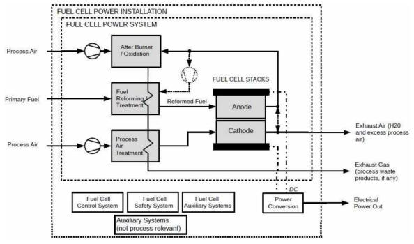
Fig 1.1 Components of Typical Fuel Cell Power Installation
